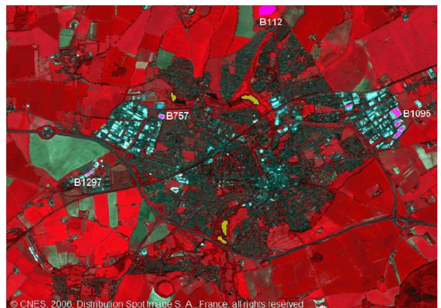
Figure 3 - Selected GCTs shown on a SPOT false colour composite. Yellow areas are selected dark targets and purple areas are selected bright targets.
