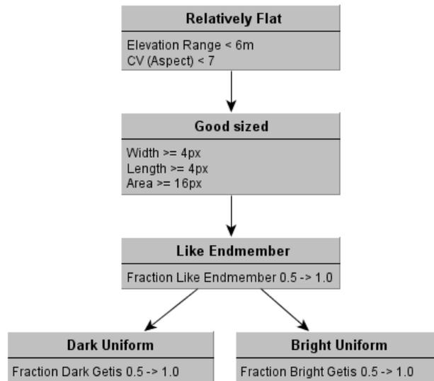
Figure 2 - Rules used for object-based classification in eCognition
